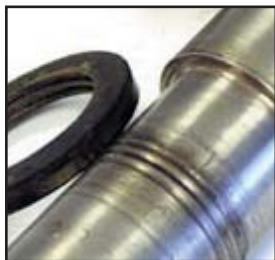
Shaft damage from a Labyrinth Seal.
