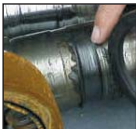
Shaft damage from a Lip Seal.
